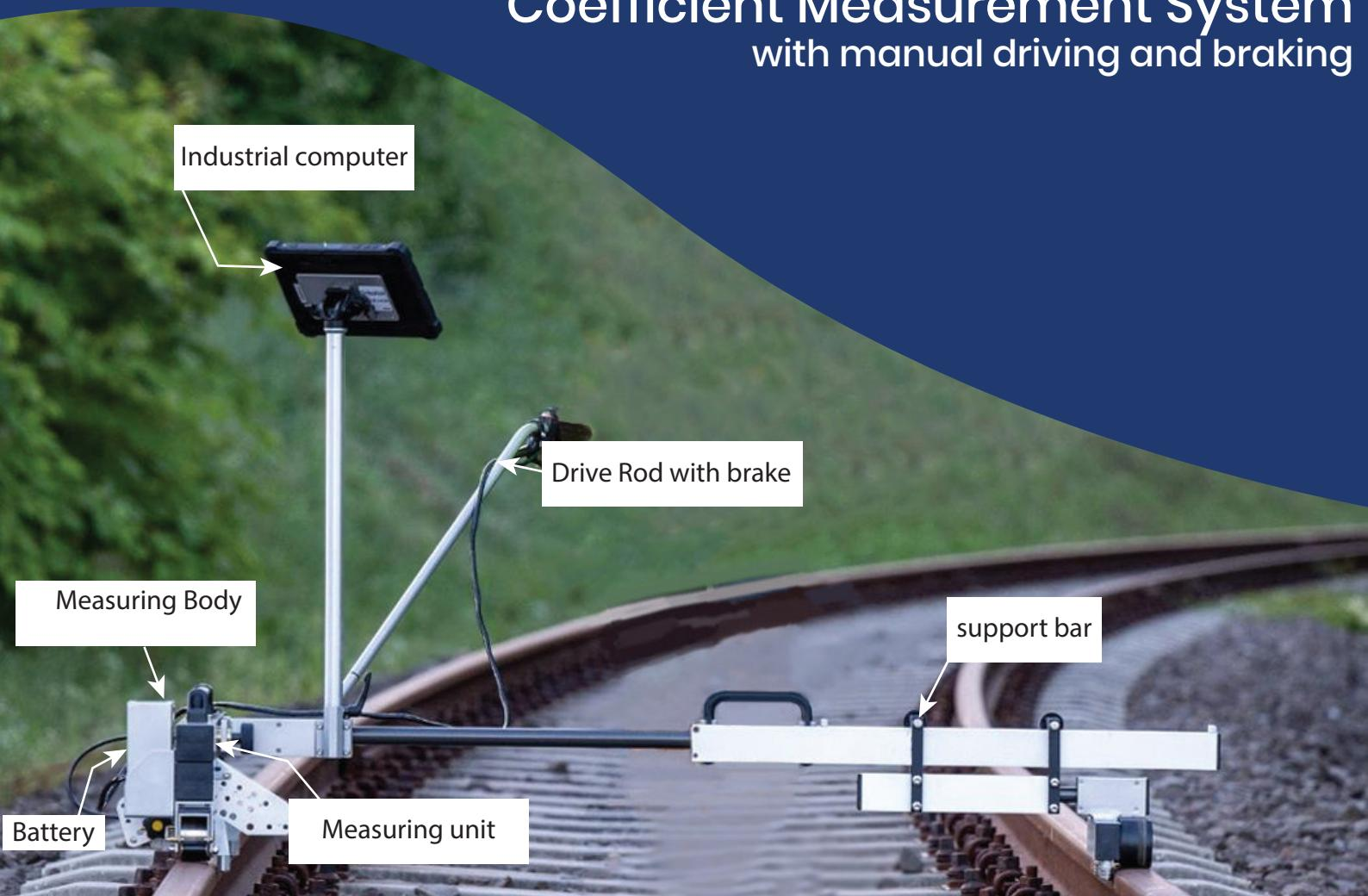
The TriboMR device was developed to measure friction coefficient that occurs between the train wheel and the rail. The TriboMR has one measuring wheel. Vertical (according to direction of movement) and normal components of force can be measured by braking this wheel and friction coefficient can be calculated with these two data. The result of this calculation is the friction coefficient between the measuring wheel and the rail.
